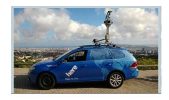
Data collection by driving with multi-cameras and LIDAR-vehicles
